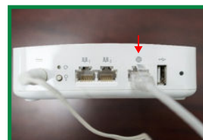
Connect ONT/fiber modem to router
